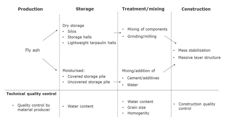
Figure 13. Brief summary of fly ash technical quality assurance during each phase in construction project
