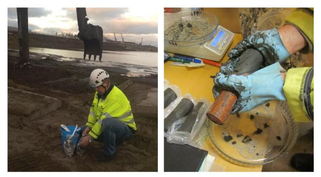
Figure 10. Sampling for environmental eligibility testing during stabilization works (left) and making of test specimens (right).
