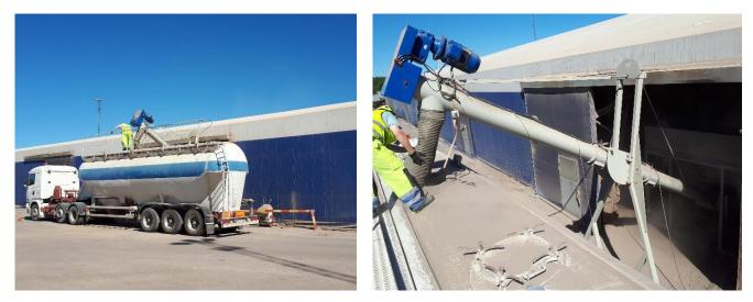
Figure 11. Tarpaulin lightweight hall can be used for dry storage of fly ash from the power plant. Dry ash is stored in hall, loaded to tank truck and transported to stabilization site.
