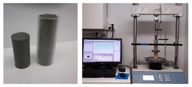
Figure 2. Stabilized test specimen (left) and UCS testing equipment (right)
